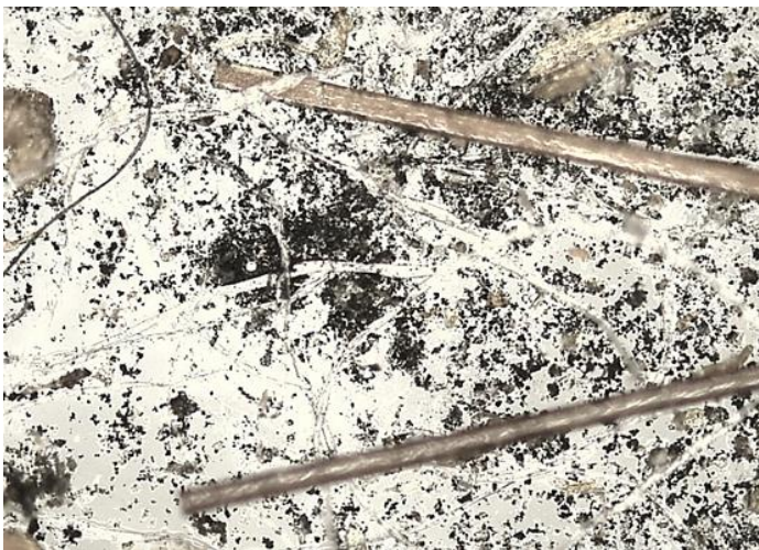
C. Structure Fire Soot Deposition (RLDF)
